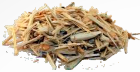
Crushed wood – e.g. as recycled 30x30 mm (40x40) fraction –moisture content up to 35%
